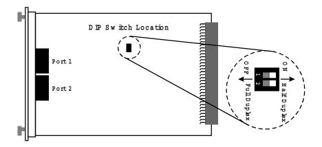
Figure 1-7. Dip switch location and mode settings
